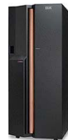
IBM p690 672CPUs 4,400GB memory 4364.8GFlops Rpeak 100TB disk
