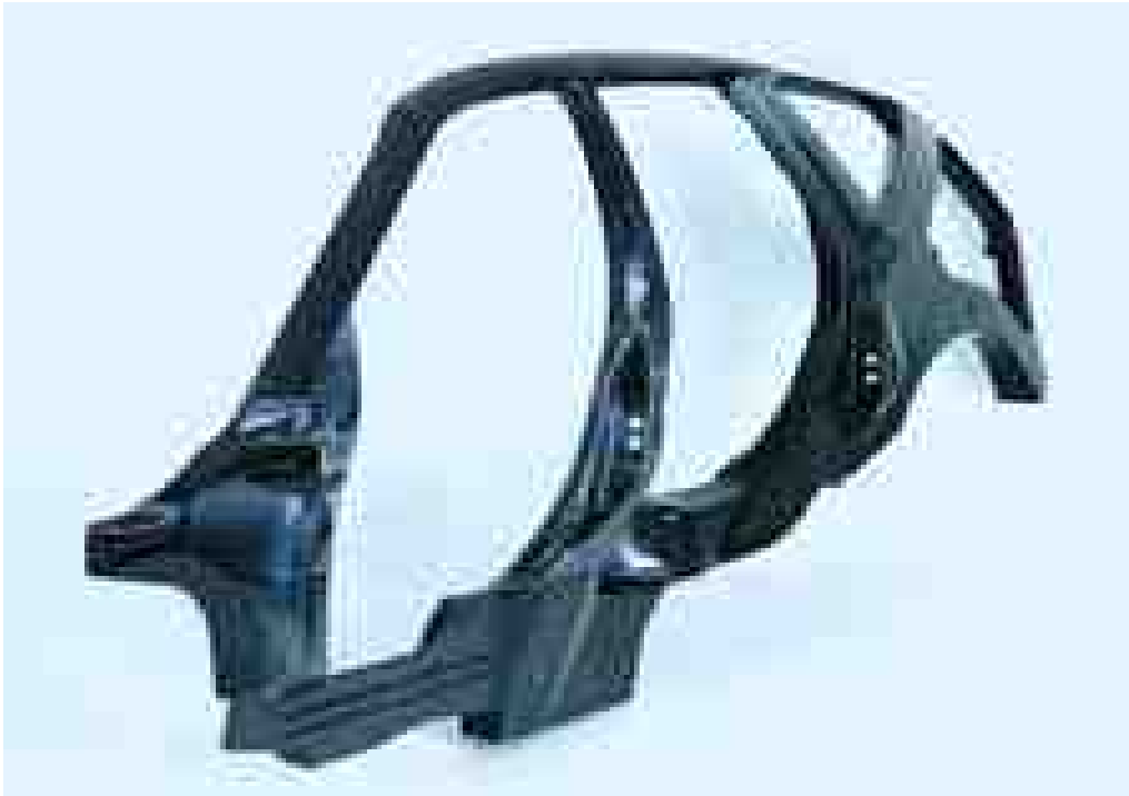
[그림 42] BMW' s Z22 CFRP side panel manufactured by RTM
